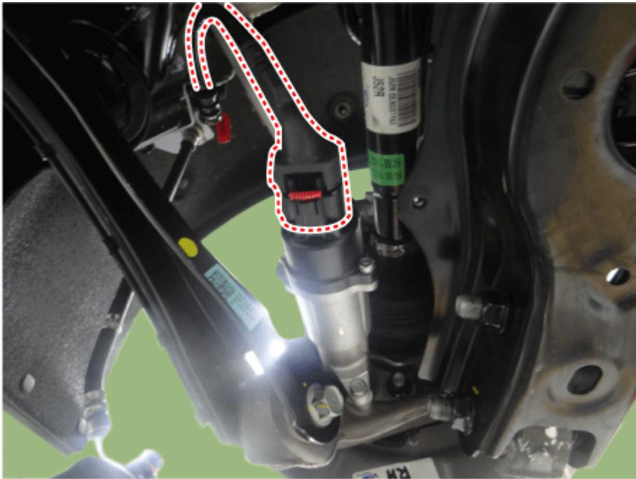
5. Loosen the EPB actuator (A) nuts and bolt (B).
