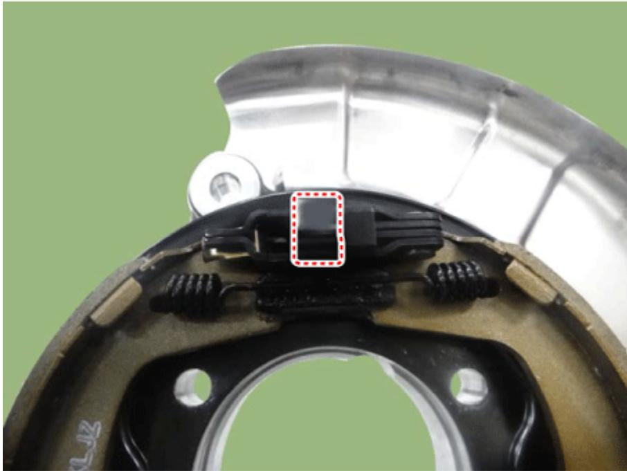
7. Using the driver, push the rod and then remove the EPB actuator.
